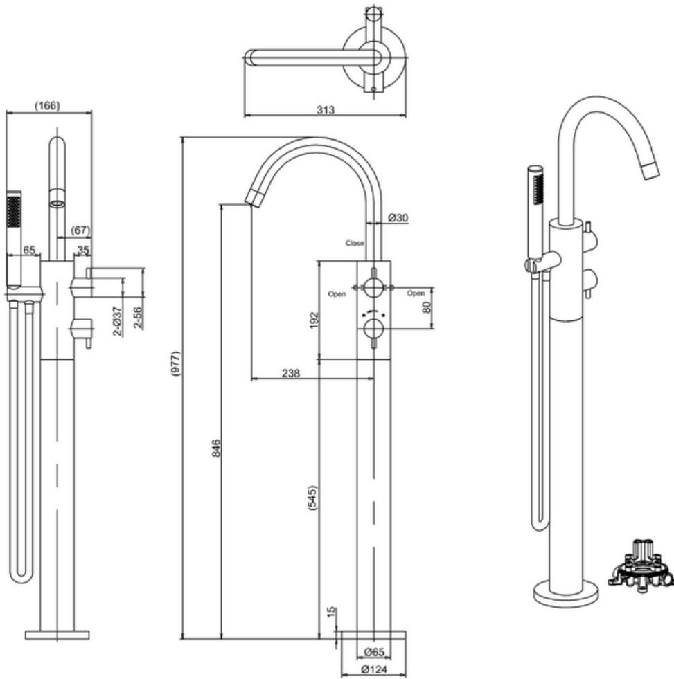
KL418TFC - Thermostatic floor standing BSM with kit
