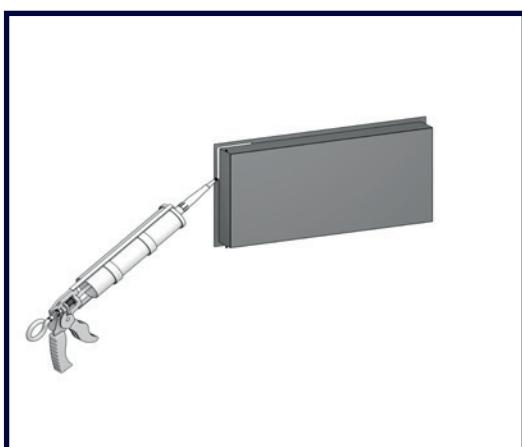
**3** apply sealant on the inside of the flange
