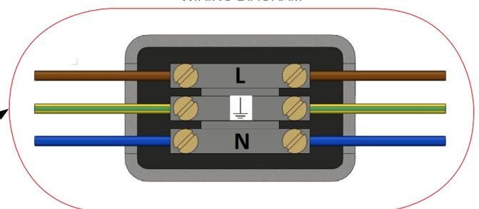
**7.** Connect the mirror wiring in an IP44 approved connector box (not included) which can be inserted into the wall anywhere behind the cabinet mirror.
