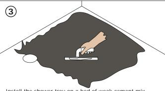
Install the shower tray on a bed of weak cement mix (sand/cement ratio 5:1). Tile adhesive can be used as an alternate to sand or cement. Please note if using water based adhesives, to enhance the bonding it is suggested that a suitable primer is applied to the base of the shower tray before installation.
