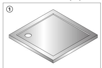
Remove protective plastic film from the areas near the waste and those sides of the tray which will be against a wall.
