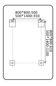
●STEP1 ●STEP2 Drill holes per drawing, then install the suckers
