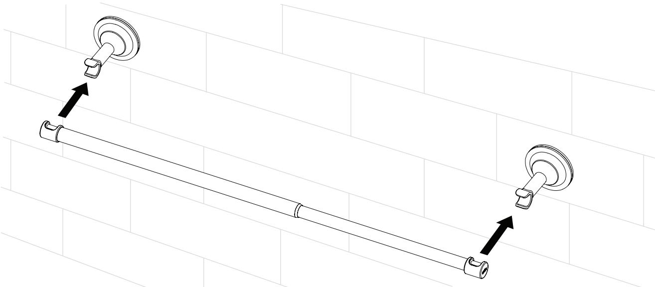
SURE-LOCK items must be mounted on smooth, non-porous surfaces like stainless steel, porcelain, tile, etc. Not for use on textured surfaces such as dry wall, quartz, marble, & stone.
