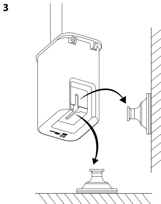
**SURE-LOCK items must be mounted on smooth, non-porous surfaces like stainless steel, porcelain, tile, etc. Not for use on textured surfaces such as dry wall, quartz, marble, & stone.**
