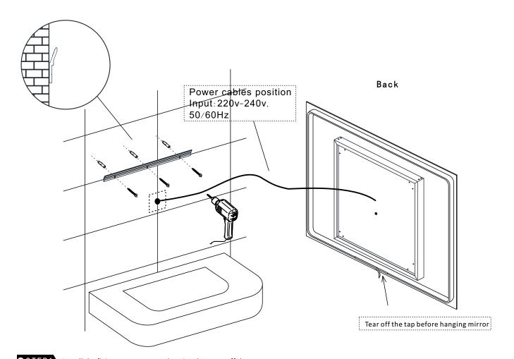
OSTEP1 Install the fixing parts, connect the wire, then tear off the tap
